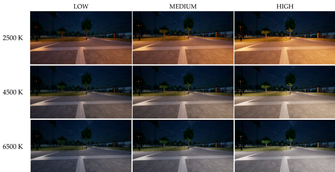
Figure 1. Matrix of the nine settings of the virtual scenario presented to participants. Rows show the three different CCT conditions. Columns show the three different overall illuminance levels.
