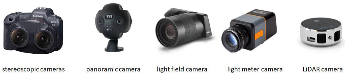
Figure 8 - Advanced cameras for physical recording and metrics in 3D space
